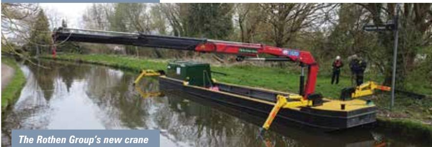
The Rothen Group's new crane boat, Oxford, carries a HMF 1120 crane, with outrigger legs
