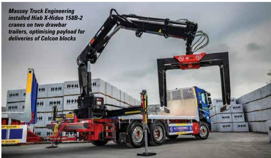
*Massey Truck Engineering installed Hiab X-Hiduo 158B-2 cranes on two drawbar trailers, optimising payload for deliveries of Celcon blocks*
