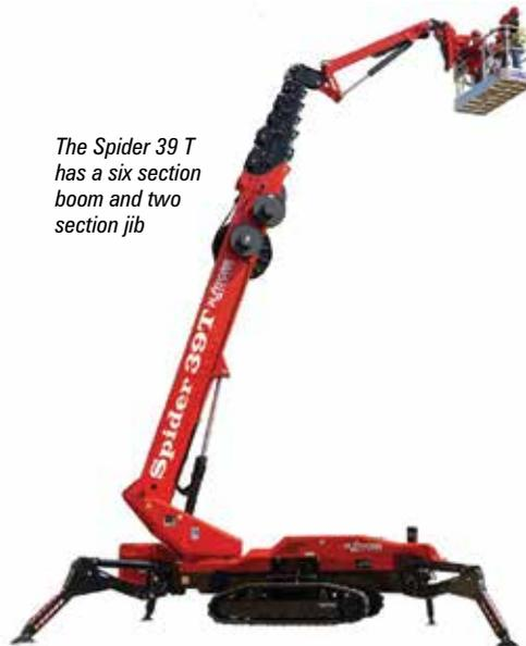
The Spider 39 T has a six section boom and two section jib
